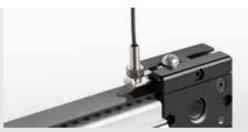
Proximity Switch M8 is a versatile device for limiting the terminal position or for reference on linear units with timing-belt drives. It is available with a permanent or plug-in connecting cable.
