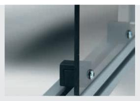
Multiblock PA is inserted into the profile groove at any position. Light cladding panels and panel elements made from Acrylic Glass, Plastic or Compound Material must be provided with a bore at the appropriate location and screwed to the Multiblock.
