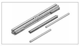
Note: Where Roller Guides are longer than 3 m, the Shafts, the Shaft-Clamp Profile and the supporting profile should be assembled with joints offset to each other.
