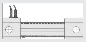
Possible arrangement of Proximity Switches 8 and Proximity-Switch Cams 8:
