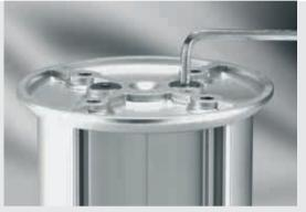
Flange 8 D130 is screwed to Column Profile D110 by means of 2 Countersunk Screws DIN 7981-M8x25. To do this, M8 threads must be tapped into the core bores ( $\varnothing$  6.8 mm) in the Column Profile.
