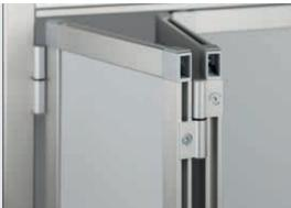
Folding-Door Hinge AI for Clamp Profile 8 32x18 is used to link together separate segments to create space-saving folding doors. Thanks to the Hinges, the moving elements fold up in a concertina formation.
