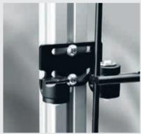
The Dual-Rod Mesh is first hung from a preassembled Dual-Rod Mesh Hanger, and then screwed into position with further Hangers. Recommended spacing of Hangers: 3 section heights, corresponding to 600 mm.
