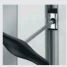
Max. torque for the tensioning screw: M = 2.5 Nm
