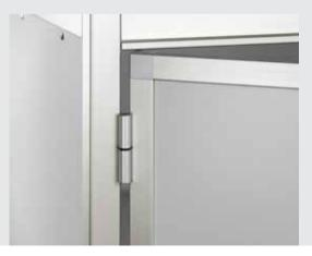
Hinge 8 Al for Clamp Profile 8 32x18 connects a frame made from Clamp Profiles 8 32x18 to a Line 8 profile. The strong door hinge is an ideal anchor for windows and folding doors.
