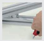
Align the CLICK-Fastening Set and tighten the tensioning
