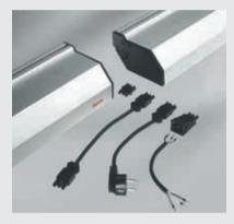
The Connecting Cable is used to connect the power supply to an earthed plug. The socket can be used to power the Light Fitting from any line network which is in place. The wires are held securely in the socket by means of a spring-force connection. If several Light Fittings are connected end-toend, the power is fed from one Light Fitting to another by means of the Adapter. The dowel which is inserted into a mounting hole in the cap provides a mechanical link between the Light Fittings.
