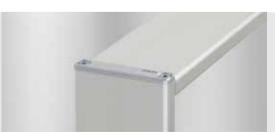
Cap 8 80x16 Zn is fixed to Profiles 8 80x16 using the enclosed screws to create a secure and friction-based connection, which ensures it can resist impacts and vibration over longterm use. A thread must be tapped into both screw channels of the flat profiles.
