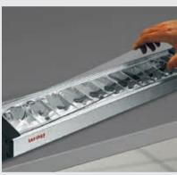
The Light Fitting can be sealed against dust (IP 40) by means of the Protective Panel. This panel also protects the Light Fitting against soiling and damage. The open socket must be sealed with a cap.
