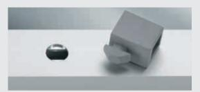
To insert Multiblock X PA in profiles with closed grooves, it is recommended to remove the groove cover at the relevant location using a counterbore. The Step Drill, Universal Connection 6 (Art. No. 0.0.431.19) is ideal for this purpose. The required counterbore depth is just 2 mm!
