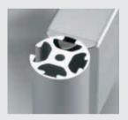
Adapters 8 D40 also serve as radial seals. In completely covering the end face of the profile, they seal the openings of the profile cross-section.
