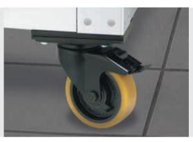
Unlike Castor D125 swivel with double-brake heavy duty, the N version allows the lock to be actuated from the trailing side. The combination of two Castors D125 swivel with double-brake and two Castors D125 swivel with double-brake N thus enables a heavy structure on swivel castors to be locked at all four castors, since the locks can always be reached easily. This prevents the structure from being moved or rolling away.
