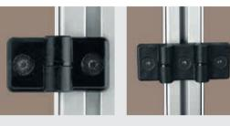
Double Hinges PA can only be used on 20 mm wide profiles in Line 5, on 30 mm wide profiles in Line 6 and on 40 mm wide profiles in Line 8.
