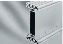
Connection Profiles 8 160 and 8 240 are supplied in pairs and machined with bores for the DIN 912-M8x60 fastening screws and DIN 934-M8 Hexagon Nuts.
