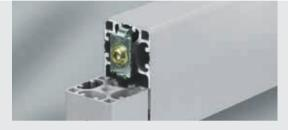
Standard-Fastening Set ESD is used in the same way as a conventional Standard-Fastening Set. The special design of the fastening screw partially destroys the insulating anodized layer on the profile groove and creates an electrical contact between the connected profiles.
