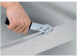
T-Slot Opener 8N is used to remove the groove cover over any length beginning from the end face of the profile or any other opening of sufficient size. If the opening does not extend to the end of the profile, the end of the opening must be defined with a hole of  $\varnothing$  9.2 mm.
