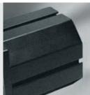
Profile 8 80x80-45° D60 is the basis for Coupling Housings 8 D30 and 8 D55, Profile 8 120x120-45° D87 is used for Coupling Housing 8 D80. The profiles can be used to produce Coupling Housings of special lengths or housings for synchronising shafts between mechanical drive elements.
