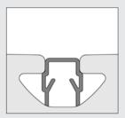
When inserted with its smooth side facing up, the Cover Profile keeps dirt and dust out of the groove.
