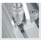
Two-part Fastener for heavy-duty securing of parts to the Profile 8 groove. The two halves of the Fastener are fitted into the groove at any point where they are then slid together. The integrated spring ball holds the Fastener in place and facilitates screw attachment.
