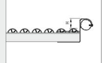
Roller Conveyor St Fastening Brackets D30 with Stop are available with different sized stops – 27 mm or 43 mm.
