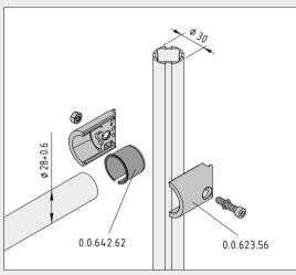
To connect an existing Tube D28 to an item Profile Tube D30, simply insert Adapter D30/D28-25 into an item Fastener D30 and the connection will hold!
