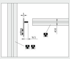
When using Profile 6 D30, an M6 thread is cut directly into the core bore.
