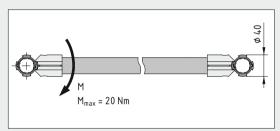
A Fastener D30 clamps Tube Adapter D30 on the Tube. Up to 4 fastening elements can be connected to one Tube Adapter D30.
