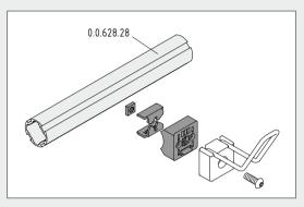
The retaining plates are used when fastening the adapter to a Line D30 Profile Tube. They use the outer profiling, hold the adapter firmly in place and are easy to position.
