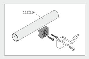
The adapter can also be fastened to Tube D30 (0.0.628.56). Self-tapping screws (0.0.644.99) are used in this case. The retaining plates must be removed from the adapter.
