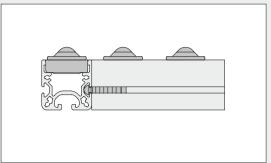
Castor Rails 8 40x40 can be interlinked using fastening elements in either the Line 5 or Line 8 grooves.
