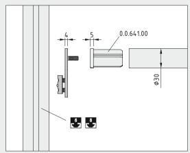
When using Tube D30 (0.0.628.56) or Profile Tube D30 (0.0.628.28), the M6 thread is provided by Threaded Insert D30 M6 (0.0.641.00).
