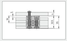
2. Fastening a panel along the length of a profile, clearance 0 and 5  $\mbox{mm}$
