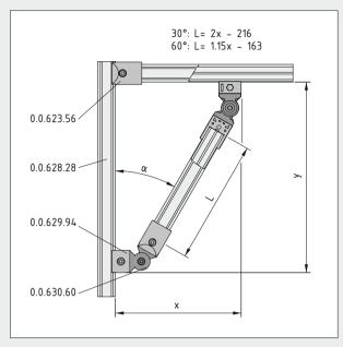
The length of connecting profile L is determined by the fastening elements that are used.
