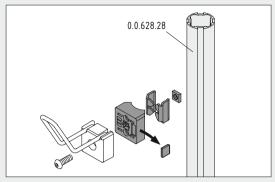
When using the adapter with vertical struts, the removable antitorsion feature must be taken out prior to assembly.
