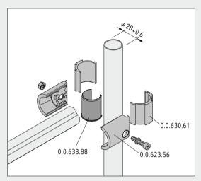
Thanks to Adapter D30/D28, it couldn't be easier to make the transition to a whole new dimension. Simply attach the Adapter to the tube ( $\varnothing$  28 mm), place a Tube Adapter D30 over it and the way is clear for extending your old structure using the innovative Line D30.
