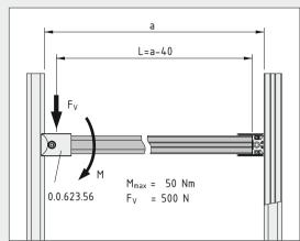
Using the Anti-Torsion Blocks makes it even easier to combine the Fastener with Profile Tubes D30 and Profiles 6 D30. They ensure the Profiles are correctly aligned in the Fastener, making it easy to avoid assembly errors.
