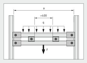
Parallel Fastener D30 connects together Profile Tubes D30, Tubes D30 (with Tube Adapter D30), Profiles 6 D30 and Profiles 8 (with Adapter 8 D30).
