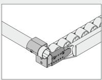
A Retaining Plate (0.0.650.83) can also be fitted to the side of guide rails e to deliver additional support. They are screwed into place using self-tapping screws driven through the upper holes in the Retaining Plate.
