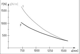
Permissible loads for profile constructions built using Tube D30, Profile Tube D30 and all variants of Profiles 6 D30.
