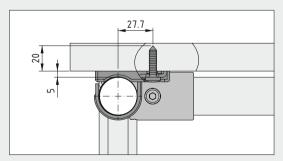
The clip is laid over the Tube D30 and fastened directly to the table top with the included screw, which is driven through the plastic spacer.
