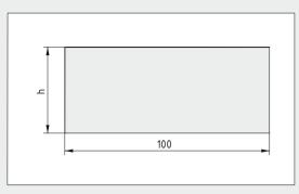
Recommended size of label cards: Label Holder D30: h = 28 mm Label Holder D30 flex: h = 42 mm
