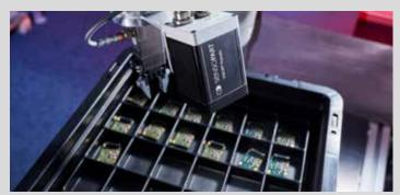
The VISOR® Robotic detects the position of the component in a load carrier and transmits the gripping position directly to the robot.
