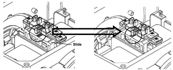
5) Connect power supply and make sure that the magnet moves centered and the air flow is OK, unplug and reassemble the pump with procedures 3) ~1).
