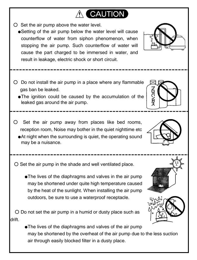
O Set the air pump in a place where working space for maintenance can be secured.
